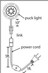
3. Link puck with power cord Secure cord to mounting surface using wire clips included.
