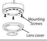
2. Attached puck to mounting surface with 3 mounting screws (included).
