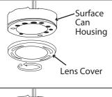
1. Remove lens cover by twisting counter-clockwise.
